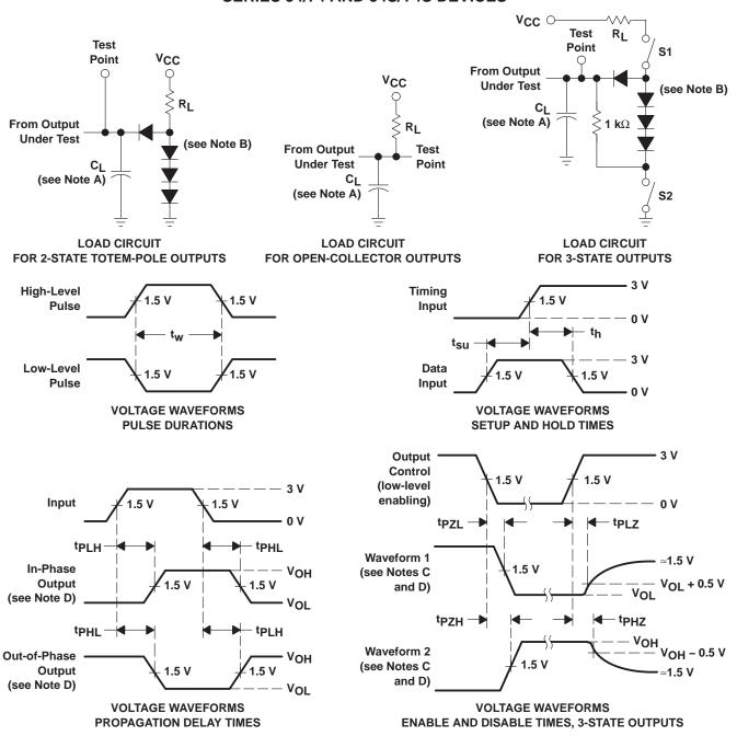
NOTES: A.  $C_L$  includes probe and jig capacitance.
