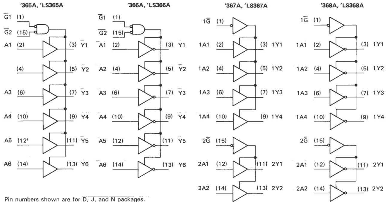
**SN54365A THRU SN54368A, SN54LS365A THRU SN54LS368A
