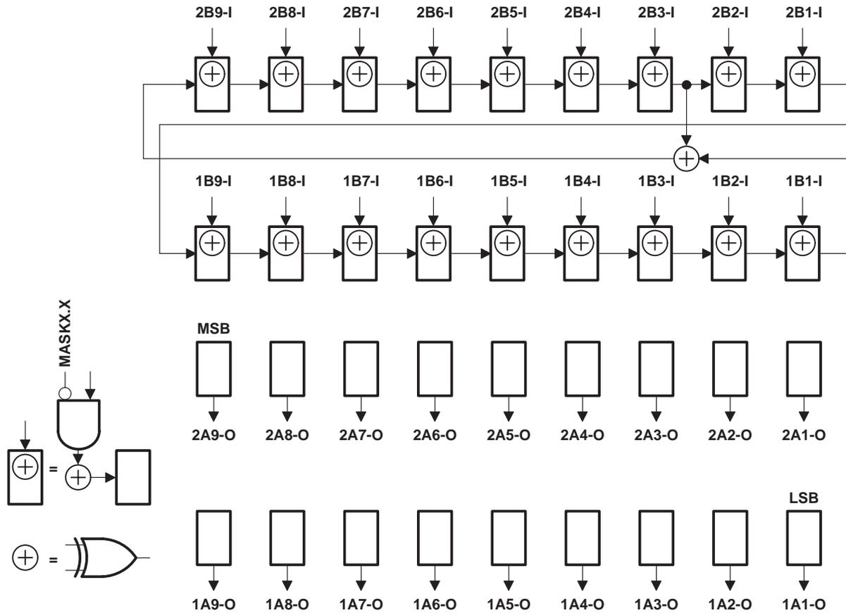
Figure 12. 18-Bit PSA/COUNT Configuration (10EA = 20EA = 1, 10EB = 20EB = 0)
