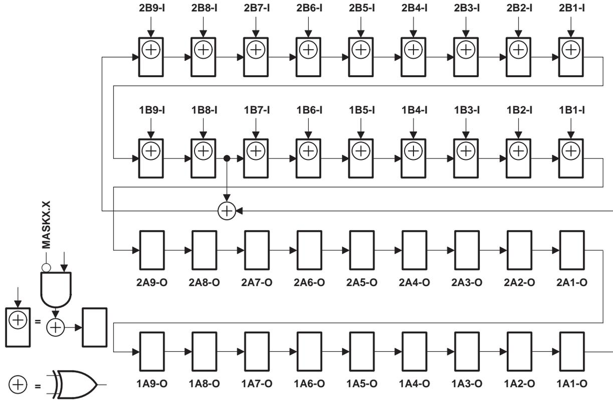
**Figure 8. 36-Bit PSA Configuration (10EA = 20EA = 1, 10EB = 20EB = 0)**
