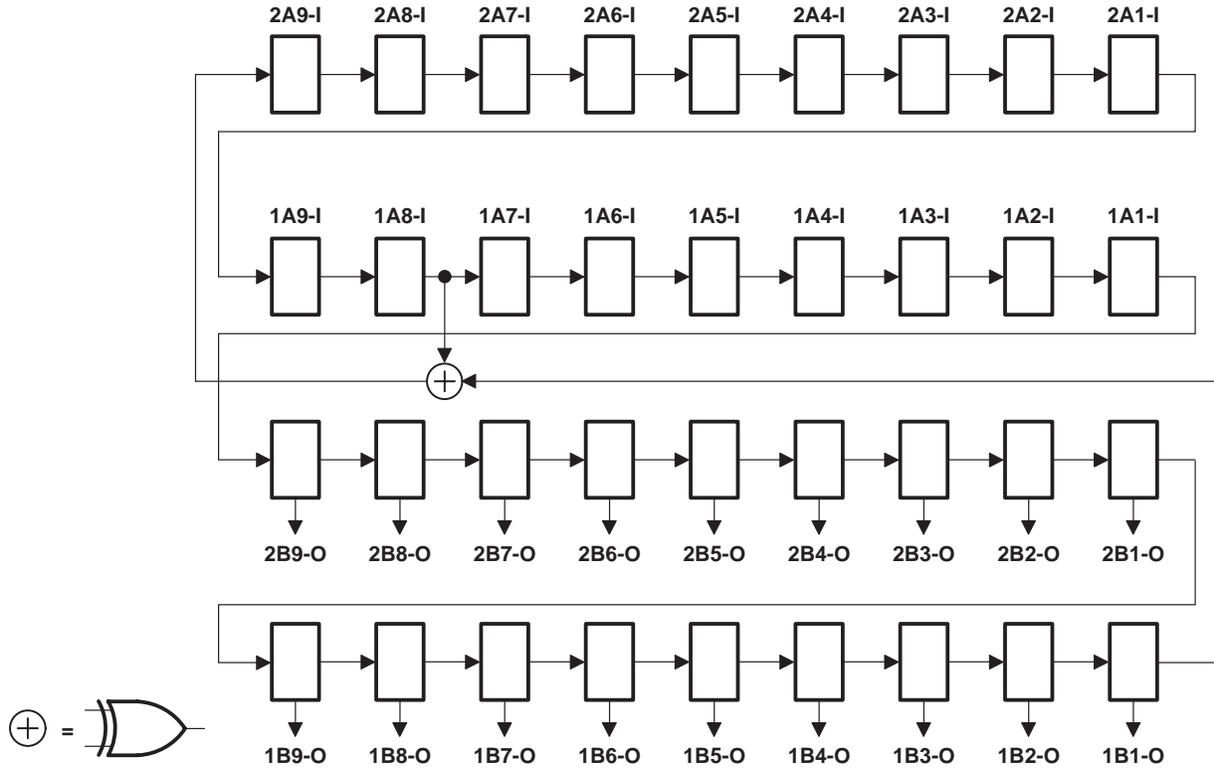
**Figure 5. 36-Bit PRPG Configuration (10EA = 20EA = 0, 10EB = 20EB = 1)**
