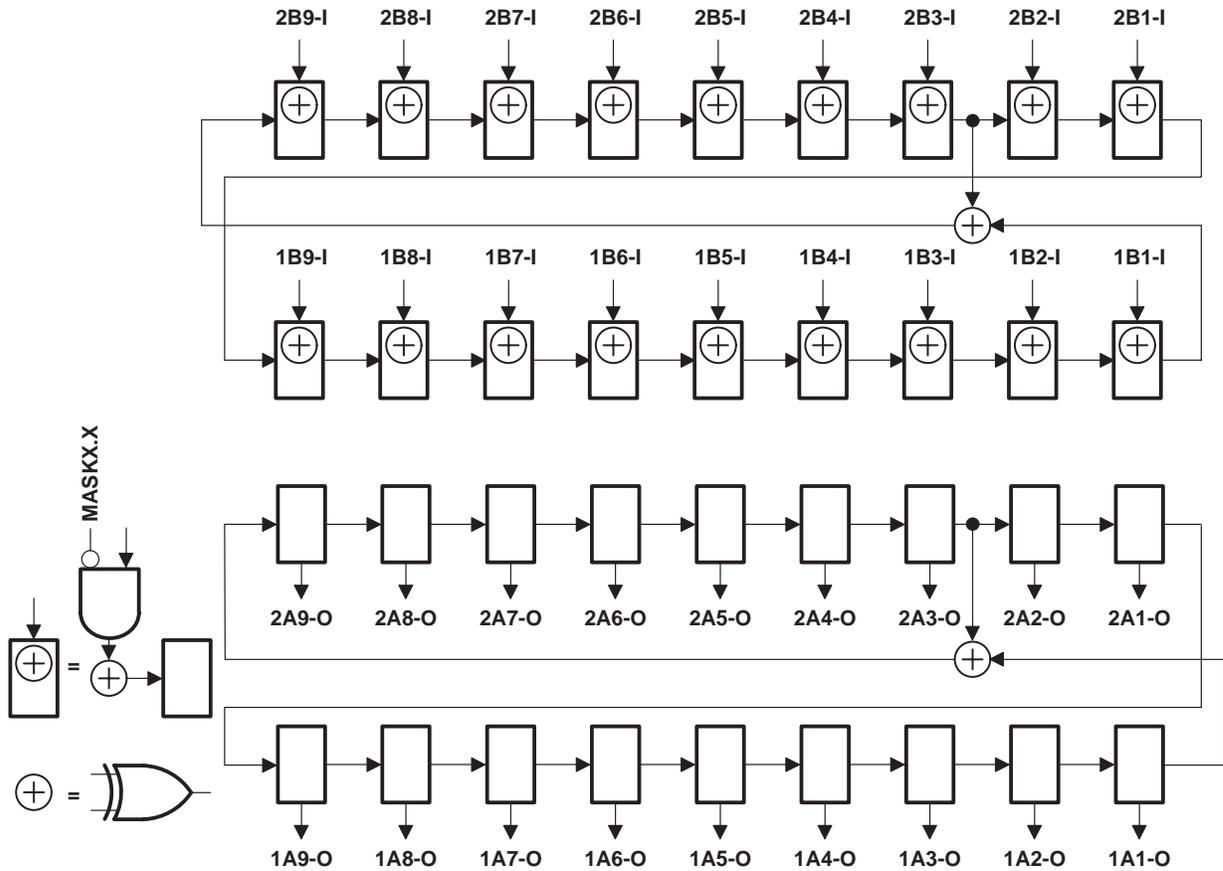
Figure 10. 18-Bit PSA/PRPG Configuration (10EA = 20EA = 1, 10EB = 20EB = 0)
