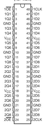
These devices can be used as two 8-bit flip-flops or one 16-bit flip-flop. On the positive transition of the clock (CLK) input, the Q outputs of the flip-flop take on the logic levels at the data (D) inputs.
