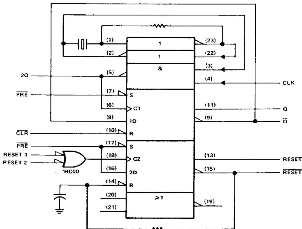
FIGURE 1. CLOCK AND RESET GENERATION FOR MICROPROCESSOR-BASED SYSTEM
