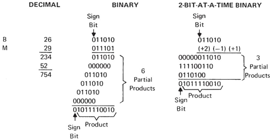
Two points should be noted in the two-bit-at-a-time-binary example above. First, in positioning the partial products beneath each other for final addition, each partial product is shifted two places to the left of the partial products above it instead of one place as is done in regular multiplication. Second, the msb of the partial product (the sign bit) is extended to the sign-bit column of the final answer.
