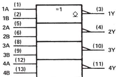
positive logic:  $Y = \overline{A \oplus B} = AB + \overline{AB}$
