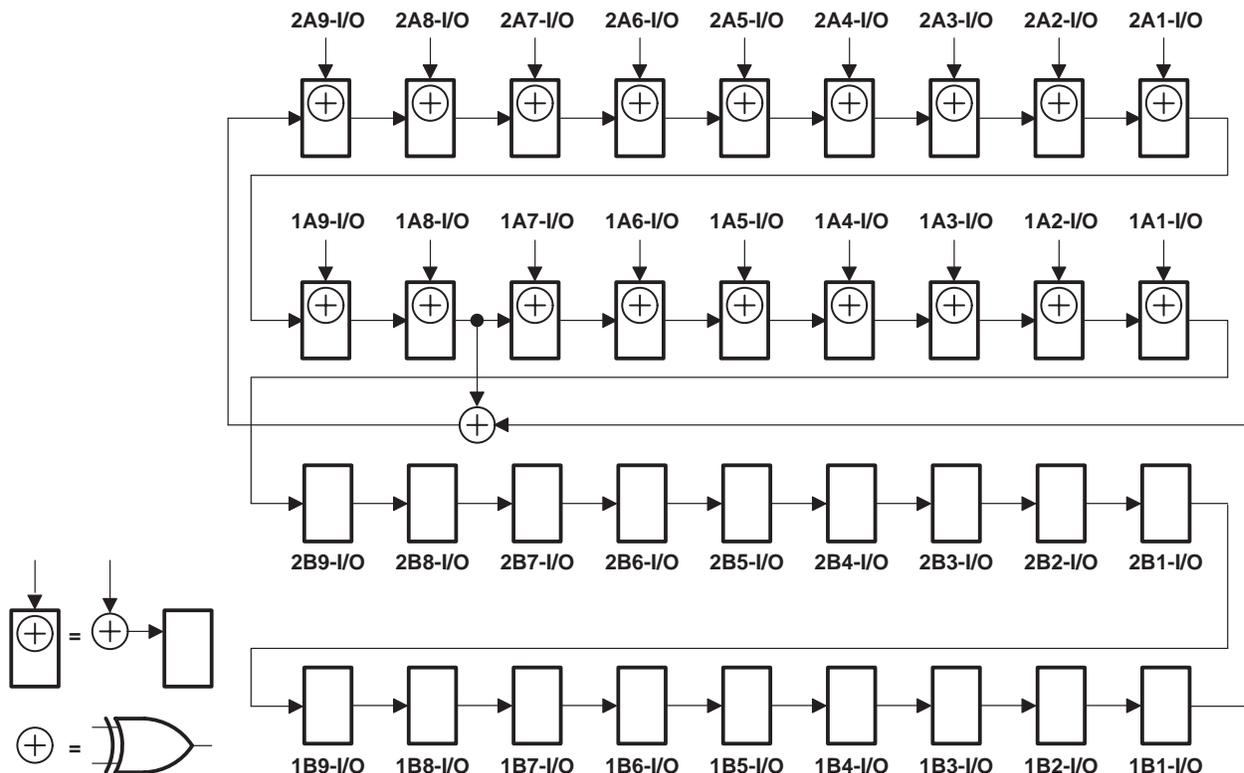
**Figure 7. 36-Bit PSA Configuration ( $\overline{1OEAB} = \overline{2OEAB} = 0$ ,  $\overline{1OEBA} = \overline{2OEBA} = 1$ )**
