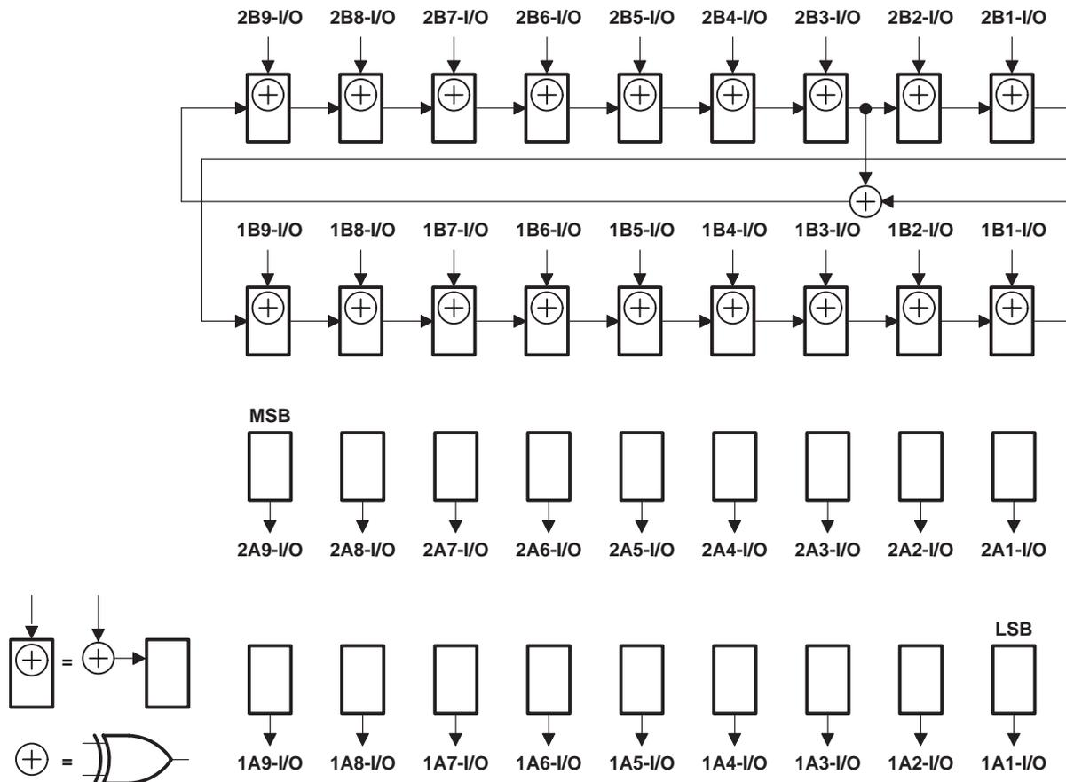
Figure 13. 18-Bit PSA/COUNT Configuration (10EA = 20EA = 1, 10EB = 20EB = 0)
