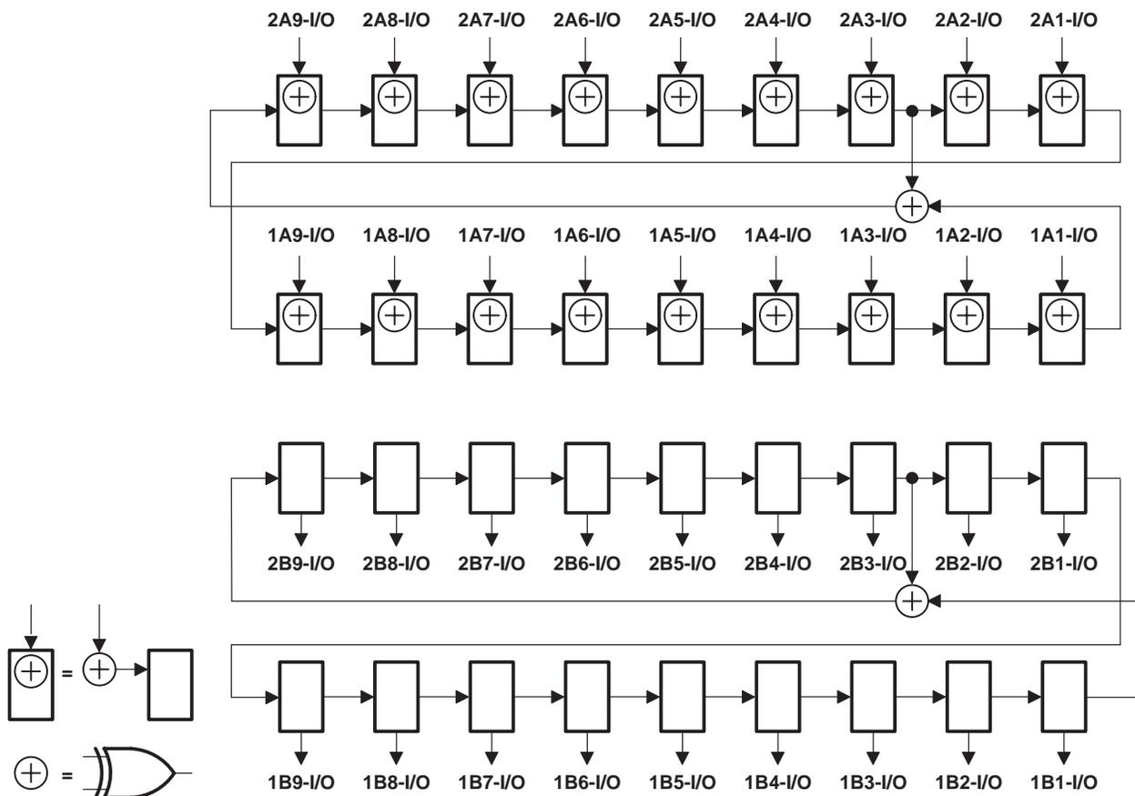
**Figure 10. 18-Bit PSA/PRPG Configuration (10EA = 20EA = 0, 10EB = 20EB = 1)**
