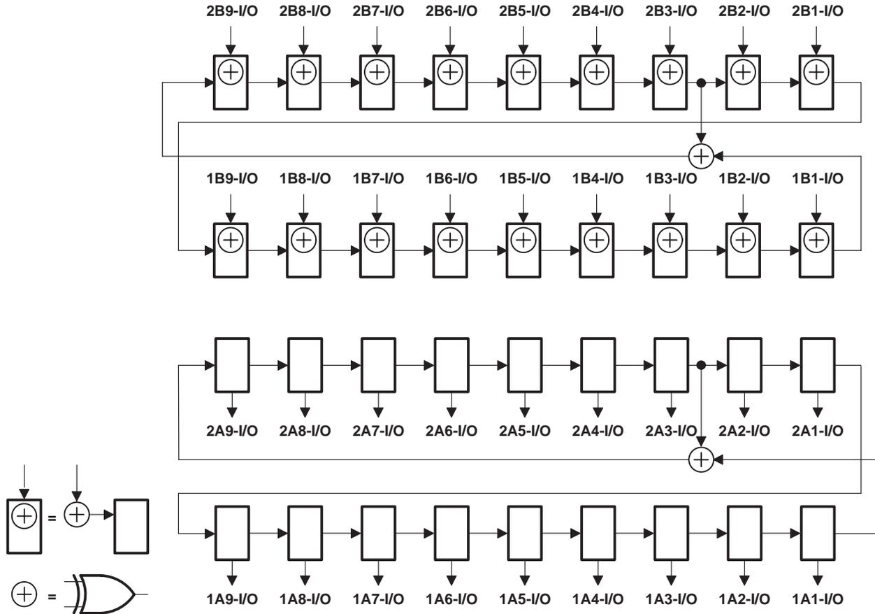
Figure 11. 18-Bit PSA/PRPG Configuration (10EA = 20EA = 1, 10EB = 20EB = 0)
