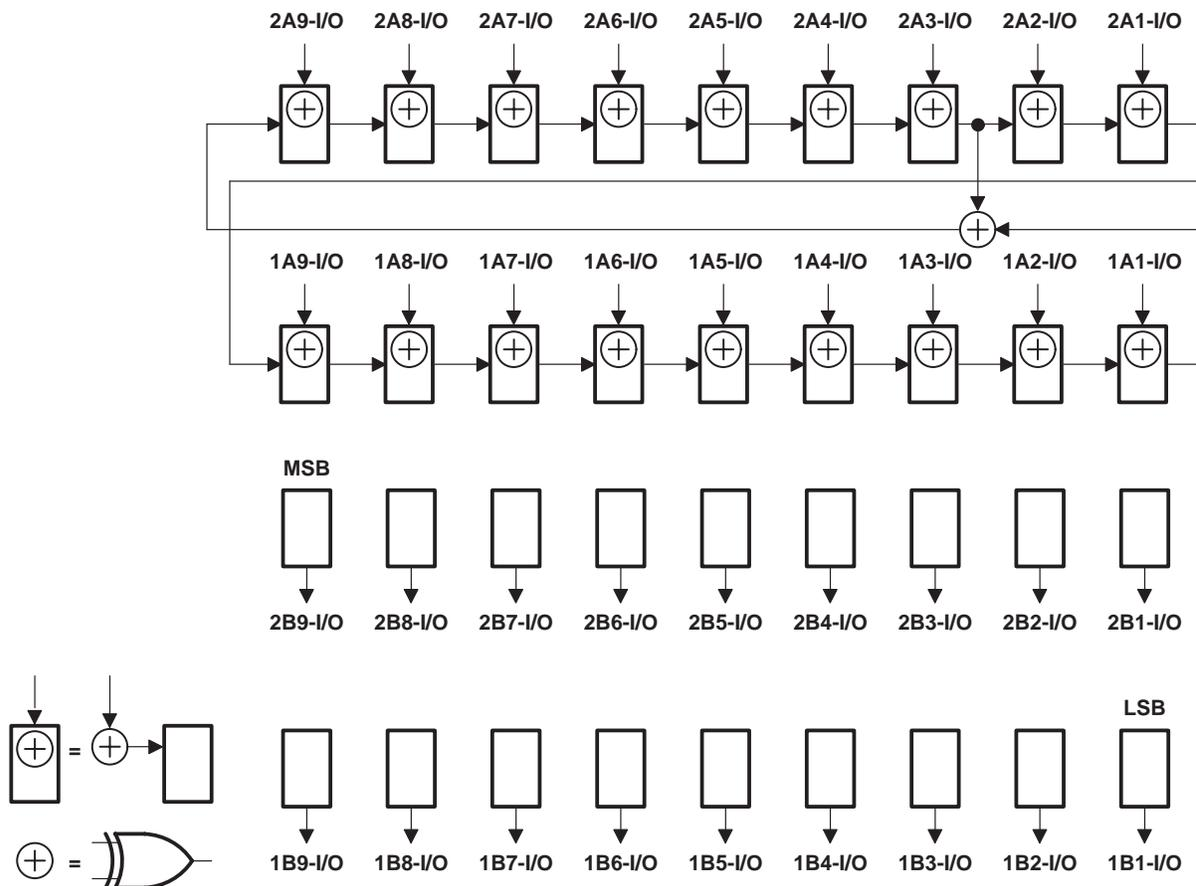
Figure 12. 18-Bit PSA/COUNT Configuration (10EA = 20EA = 0, 10EB = 20EB = 1)
