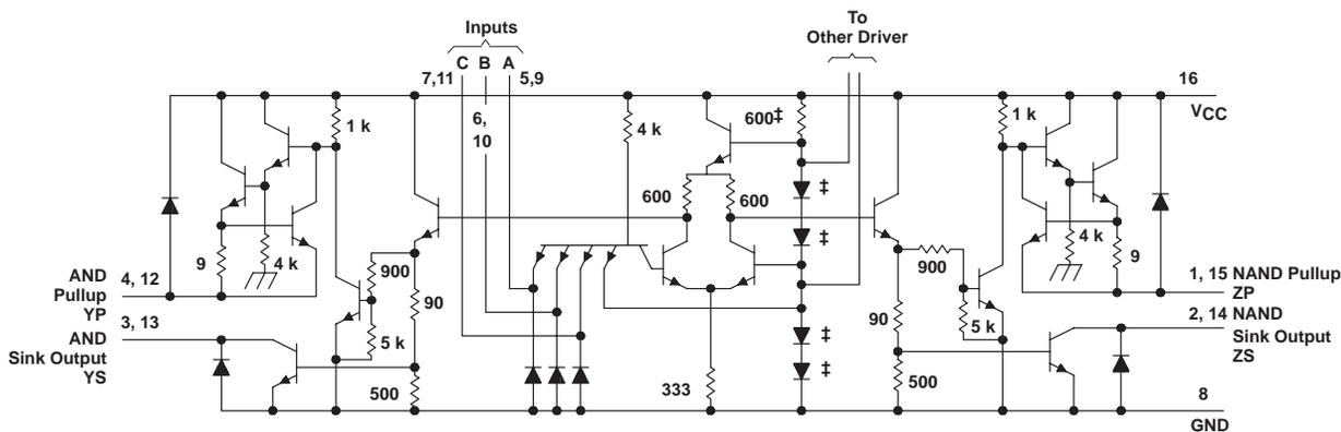
‡ These components are common to both drivers. Resistor values shown are nominal and in ohms.
