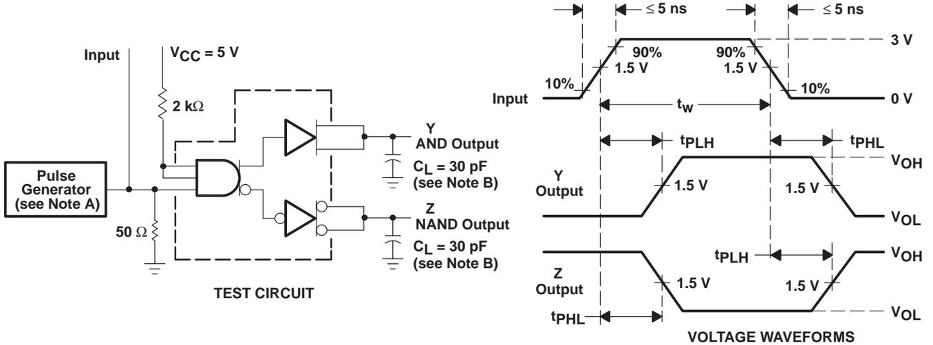
NOTES: A. The pulse generator has the following characteristics:  $Z_O = 500 \Omega$ ,  $PRR \leq 500 \text{ kHz}$ ,  $t_w \leq 100 \text{ ns}$ .
