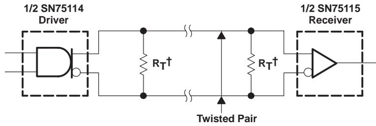
$^\dagger R_T = Z_0$ . A capacitor can be connected in series with  $R_T$  to reduce power dissipation.
