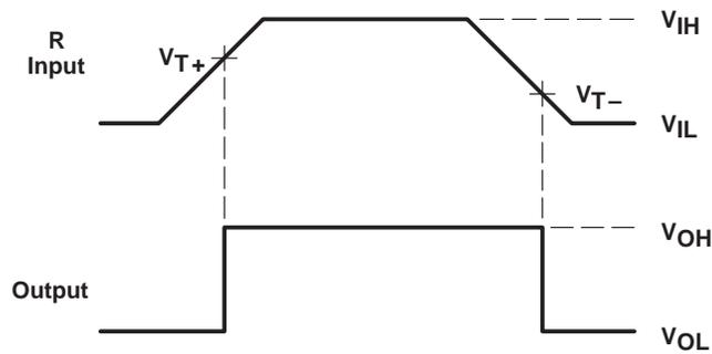
NOTE: The high gain and built-in hysteresis of the SN55122 and SN75122 line receivers enable them to be used as Schmitt triggers in squaring pulses.
