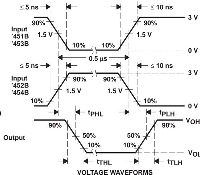
NOTES: A. The pulse generator has the following characteristics: PRR ≤ 1 MHz, Z<sub>O</sub> = 50 Ω.
