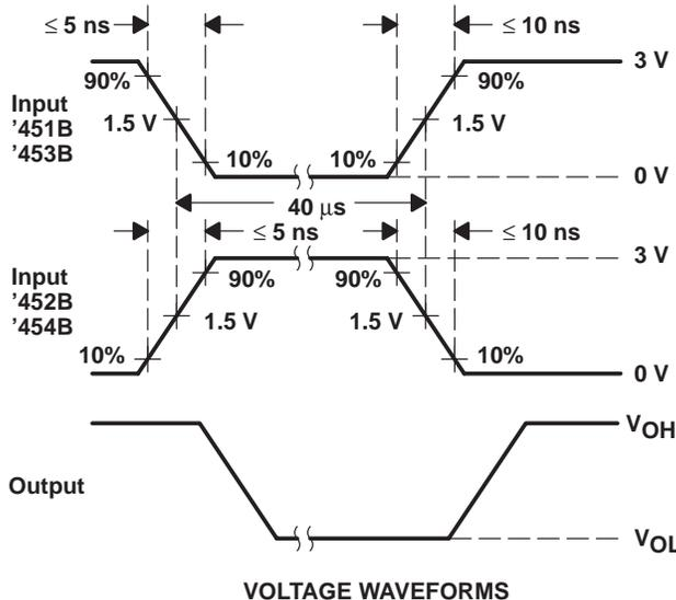
NOTES: A. The pulse generator has the following characteristics: PRR ≤ 12.5 kHz, Z<sub>O</sub> = 50 Ω.
