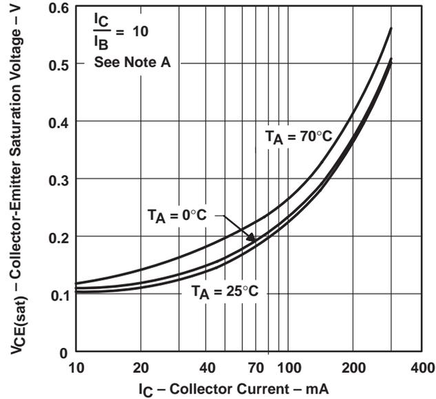
NOTE A: These parameters must be measured using pulse techniques,  $t_w = 300 \mu\text{s}$ , duty cycle  $\leq 2\%$ .
