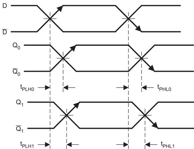
$$\text{Device Skew} = [(t_{PLH1} - t_{PLH0}), (t_{PHL1} - t_{PHL0})]$$
