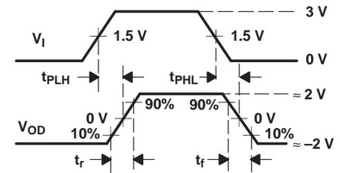
Generator: PRR = 500 kHz, 50% Duty Cycle,  $t_r < 6$  ns,  $t_f < 6$  ns,  $Z_O = 50 \Omega$
