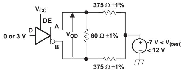
Figure 2. Driver  $V_{OD}$  With Common-Mode Loading Test Circuit
