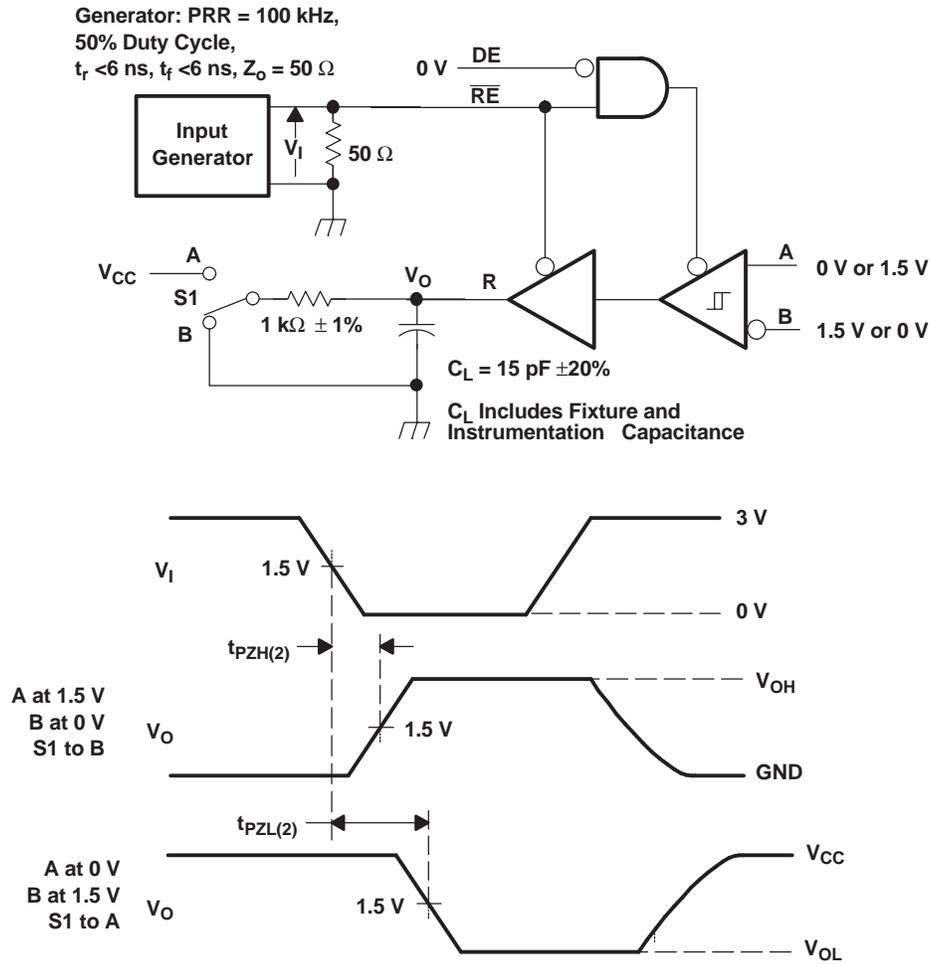
Figure 10. Receiver Enable Time From Standby (Driver Disabled)
