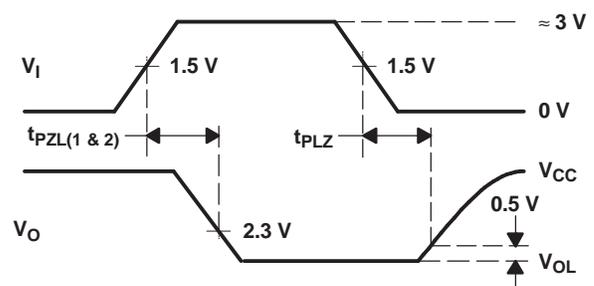
Generator: PRR = 100 kHz, 50% Duty Cycle,  $t_r < 6$  ns,  $t_f < 6$  ns,  $Z_O = 50 \Omega$
