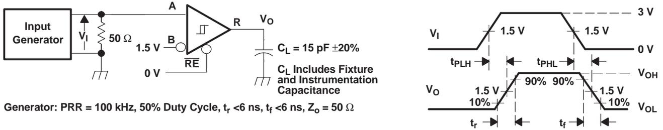
Figure 8. Receiver Switching Test Circuit and Voltage Waveforms
