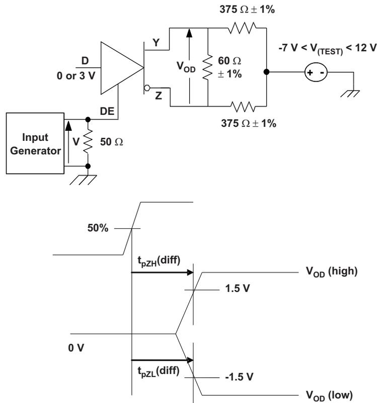
Figure 24. Driver Enable Time From DE to  $V_{\text{OD}}$
