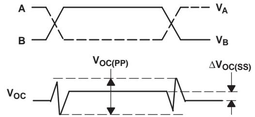
Input: PRR = 500 kHz, 50% Duty Cycle,  $t_r < 6$  ns,  $t_f < 6$  ns,  $Z_O = 50 \Omega$
