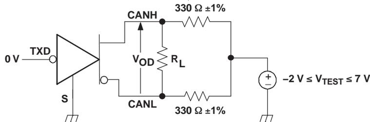
Figure 3. Driver V<sub>OD</sub> Test Circuit
