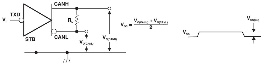
NOTE: All  $V_1$  input pulses are from 0 V to  $V_{CC}$  and supplied by a generator having the following characteristics:  $t_r$  or  $t_f \leq 6$  ns, pulse repetition rate (PRR) = 125 kHz, 50% duty cycle.
