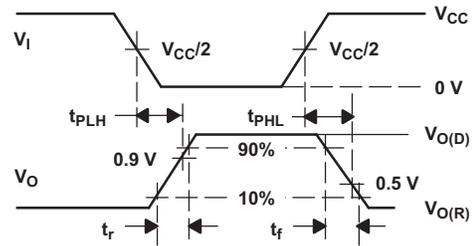
Figure 4. Driver Test Circuit and Voltage Waveforms
