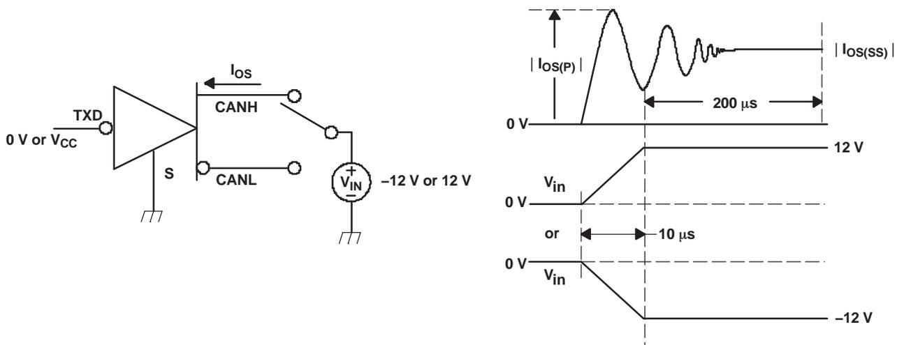
Figure 11. Driver Short-Circuit Current Test and Waveforms
