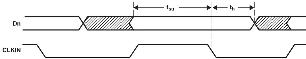
A. All input timing is defined at 1.4 V on an input signal with a 10%-to-90% rise or fall time of less than 5 ns.
