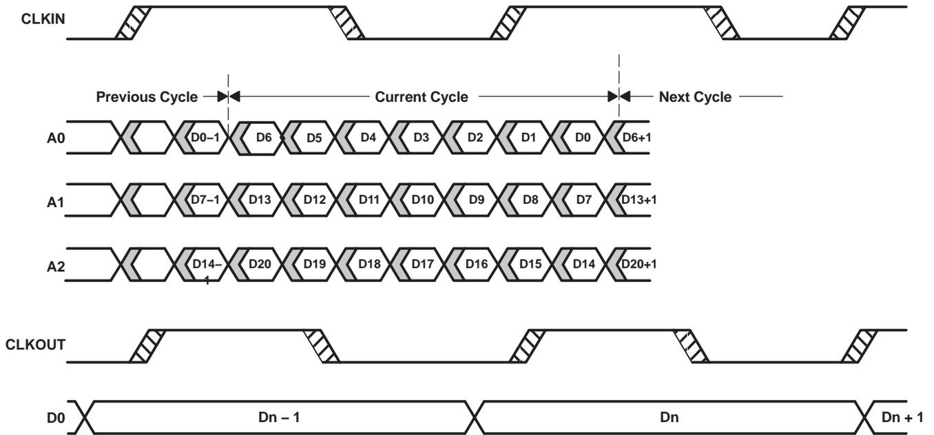
Figure 1. SN65LVDS86A Load and Shift Timing Sequences
