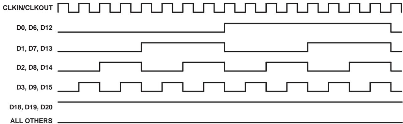
A. The 16-grayscale test-pattern test device power consumption for a typical display pattern.
