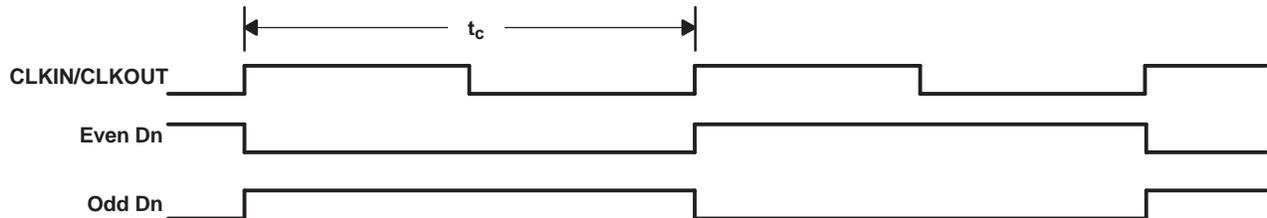
A. The worst-case test pattern produces nearly the maximum switching frequency for all of the LVTTTL outputs.
