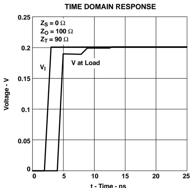
Figure 15. High-Source Impedance
