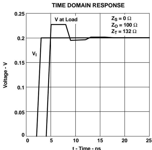
Figure 14. Low-Source Impedance
