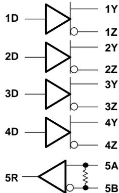
**SN65LVDT14 LOGIC DIAGRAM (POSITIVE LOGIC)**
