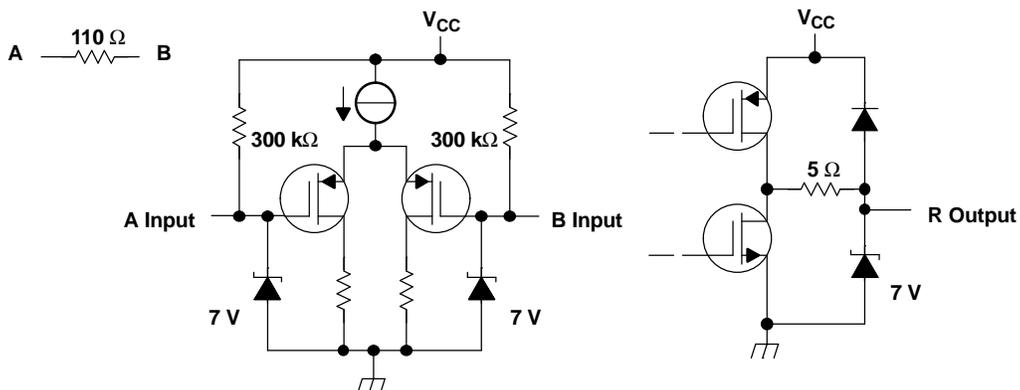
DRIVER EQUIVALENT INPUT AND OUTPUT SCHEMATIC DIAGRAMS
