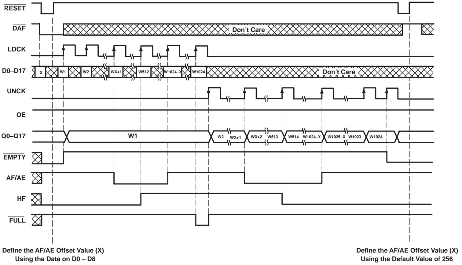
Figure 1. Write, Read, and Flag Timing Reference
