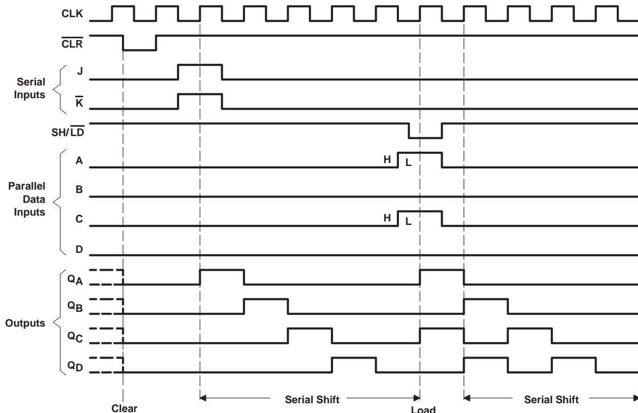
Figure 1. Typical Clear, Shift, and Load Sequences
