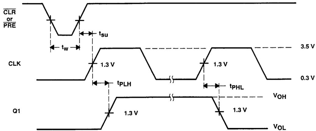
**Figure 1. Load Circuit and Voltage Waveforms**
