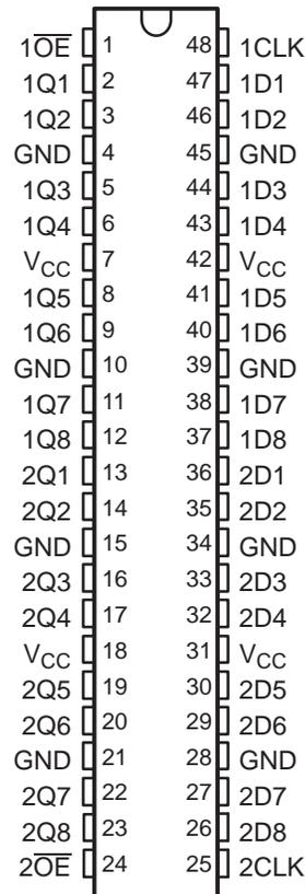
The SN74AUCH16374 is particularly suitable for implementing buffer registers, I/O ports, bidirectional bus drivers, and working registers. It can be used as two 8-bit flip-flops or one 16-bit flip-flop. On the positive transition of the clock (CLK) input, the Q outputs of the flip-flop take on the logic levels set up at the data (D) inputs.
