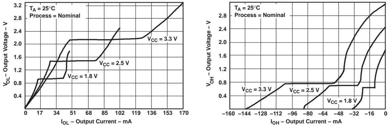
Figure 1. Typical Output Voltage vs Output Current
