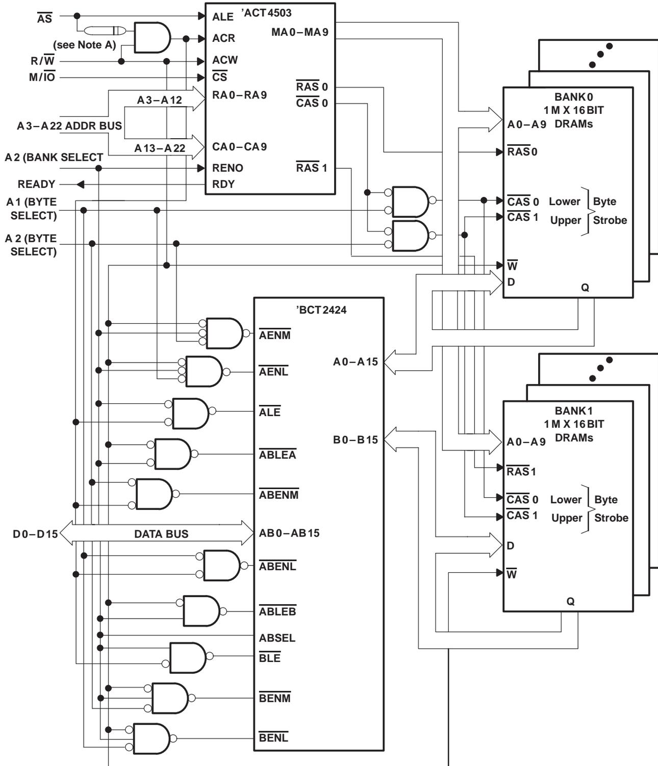
NOTE A: The value of this delay element is dependent on the speed of the microprocessor.
