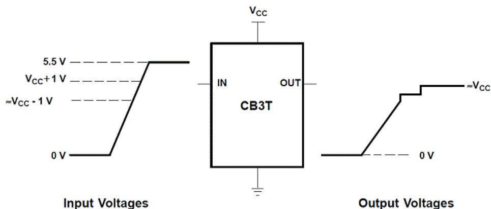
If the input high voltage (V<sub>IH</sub>) level is greater than or equal to V<sub>CC</sub> + 1V, and less than or equal to 5.5 V, the output high voltage (V<sub>OH</sub>) level will be equal to approximately the V<sub>CC</sub> voltage level.
