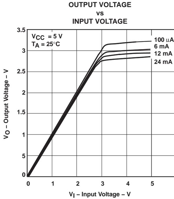
**Figure 5. Data Output Voltage vs Data Input Voltage**
