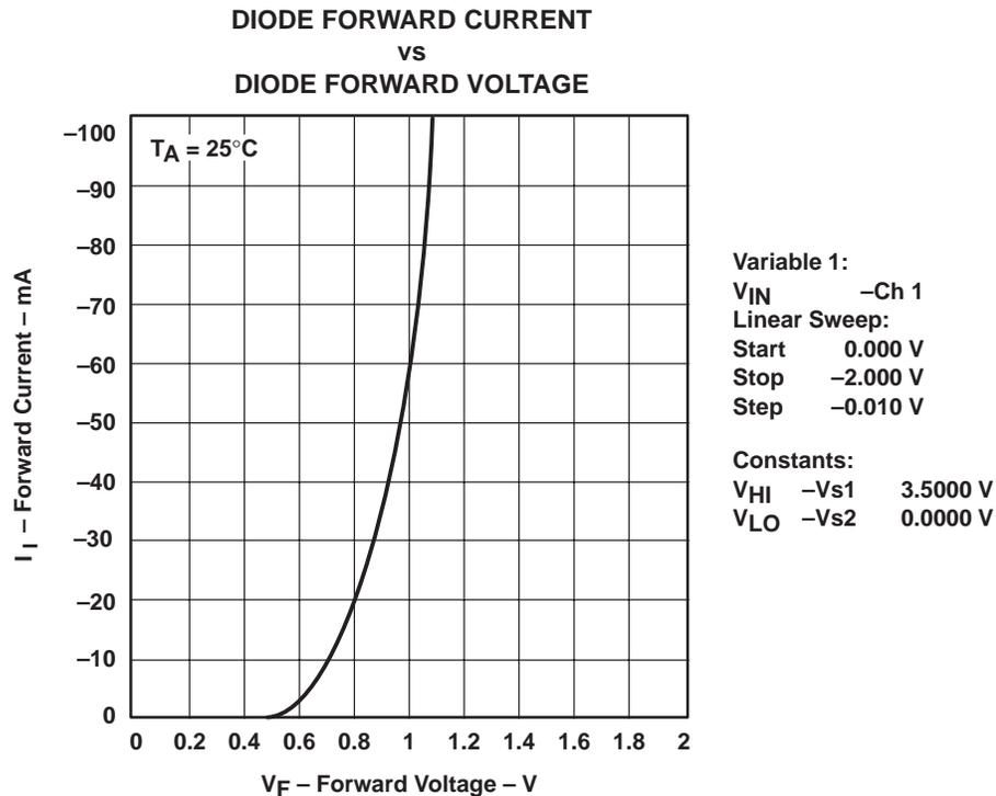
**Figure 1. Current Versus Voltage for the SN74F1056**
