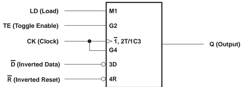
logic diagram, each D/T flip-flop (positive logic)
