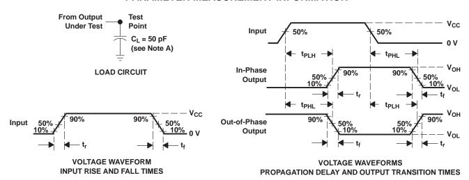
NOTES: A. C<sub>L</sub> includes probe and test-fixture capacitance.
