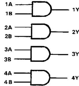
$$Y = A \cdot B \text{ or } Y = \overline{\overline{A} + \overline{B}}$$
