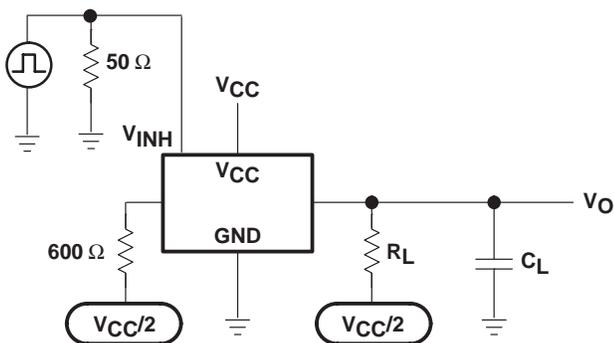
**Figure 8. Crosstalk Between Control Input and Switch Output**
