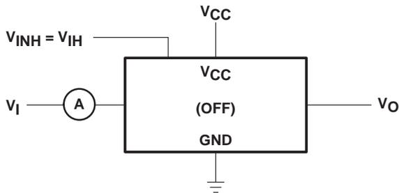
Condition 1:  $V_I = 0, V_O = V_{CC}$
