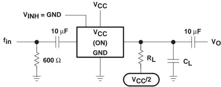
Figure 10. Sine-Wave Distortion
