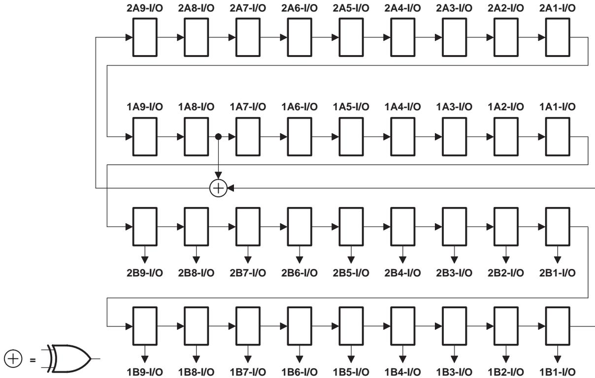
**Figure 5. 36-Bit PRPG Configuration ( $\overline{1OEAB} = \overline{2OEAB} = 0$ ,  $\overline{1OEBA} = \overline{2OEBA} = 1$ )**
