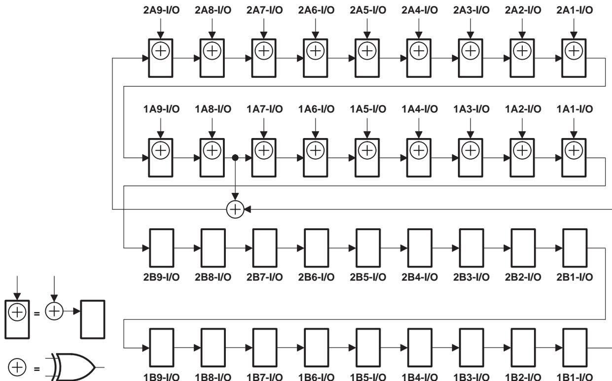
**Figure 7. 36-Bit PSA Configuration ( $\overline{1OEAB} = \overline{2OEAB} = 0$ ,  $\overline{1OEBA} = \overline{2OEBA} = 1$ )**
