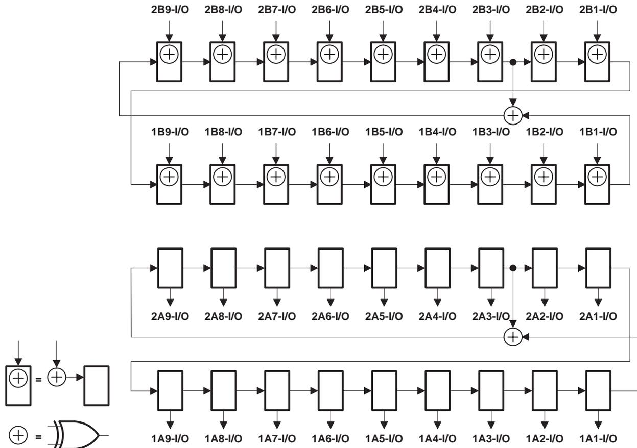
**Figure 10. 18-Bit PSA/PRPG Configuration ( $\overline{1OEAB} = \overline{2OEAB} = 1$ ,  $\overline{1OEBA} = \overline{2OEBA} = 0$ )**
