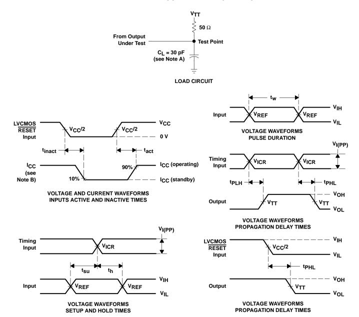
NOTES: A.  $C_L$  includes probe and jig capacitance.
