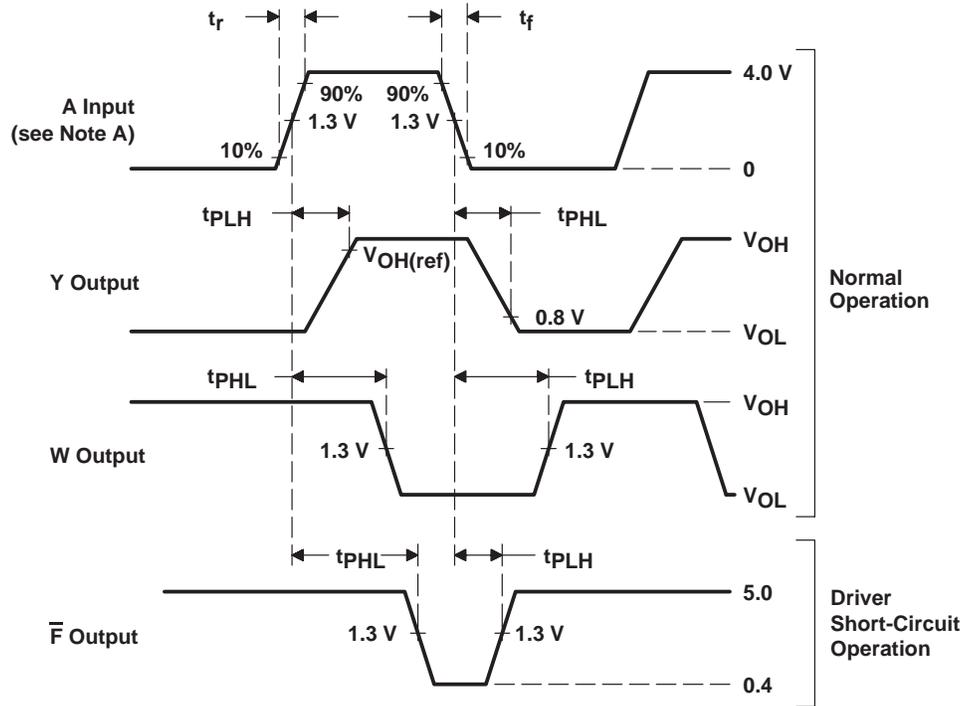
NOTE A: The input pulse is supplied by a generator having the following characteristics: PRR = 1 MHz, duty cycle = 50%,  $t_r \leq 6$  ns,  $t_f \leq 6$  ns,  $Z_O = 50 \Omega$ .
