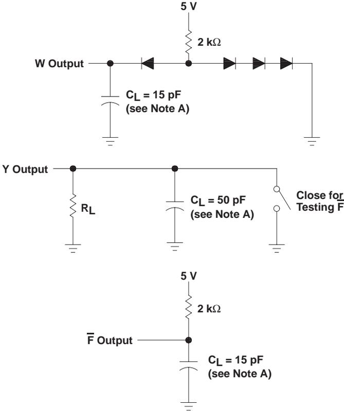
NOTE A:  $C_L$  includes probe and stray capacitance.
