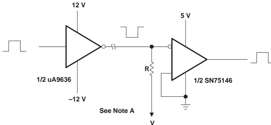
NOTE A: In order to meet the input-impedance and open-circuit-input voltage requirements of ANSI Standard EIA/TIA-232-E and ITU recommendation V.28 and ensure open-circuit-input fail-safe operation, R and V are selected to satisfy the following equations:
