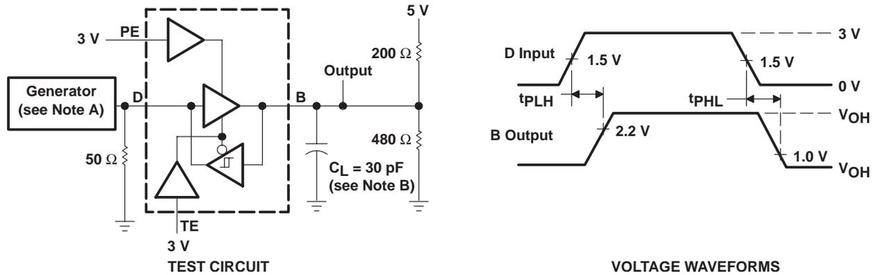
**Figure 1. Terminal-to-Bus Test Circuit and Voltage Waveforms**
