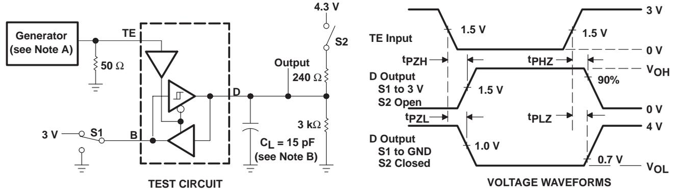
Figure 4. TE-to-Terminal Test Circuit and Voltage Waveforms
