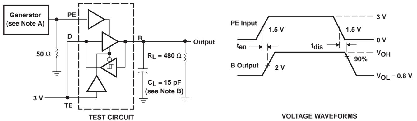
Figure 5. PE-to-Bus Pullup Test Circuit and Voltage Waveforms
