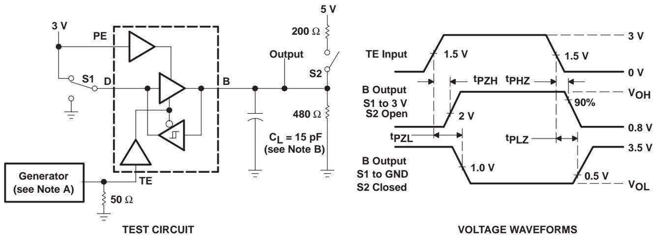
**Figure 3. TE-to-Bus Test Circuit and Voltage Waveforms**
