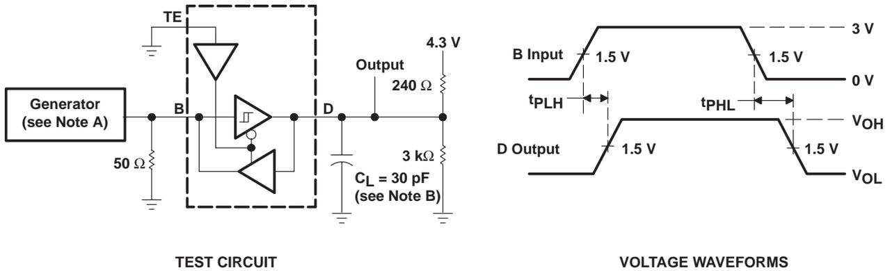
**Figure 2. Bus-to-Terminal Test Circuit and Voltage Waveforms**
