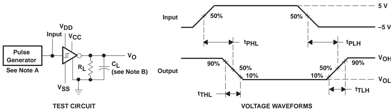
NOTES: A. The pulse generator has the following characteristics:  $t_w = 25 \mu s$ ,  $PRR = 20 \text{ kHz}$ ,  $Z_O = 50 \Omega$ ,  $t_r = t_f < 50 \text{ ns}$ .
