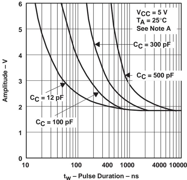
NOTE A: This figure shows the maximum amplitude of a positive-going pulse that, starting from 0 V, does not cause a change of the output level.
