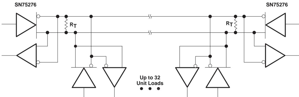
NOTE A: The line should be terminated at both ends in its characteristic impedance. Stub lengths off the main line should be kept as short as possible ( $R_T = Z_0$ ).
