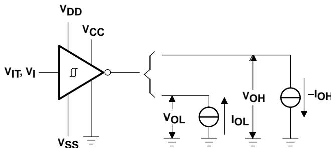
Figure 5. Receiver Test Circuit ( $V_{IT}$ ,  $V_{OL}$ ,  $V_{OH}$ )
