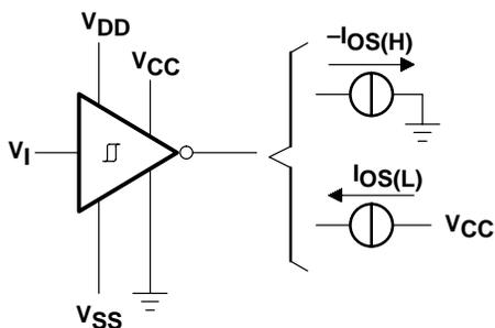
Figure 4. Receiver Test Circuit ( $I_{OSH}$ ,  $I_{OL}$ )
