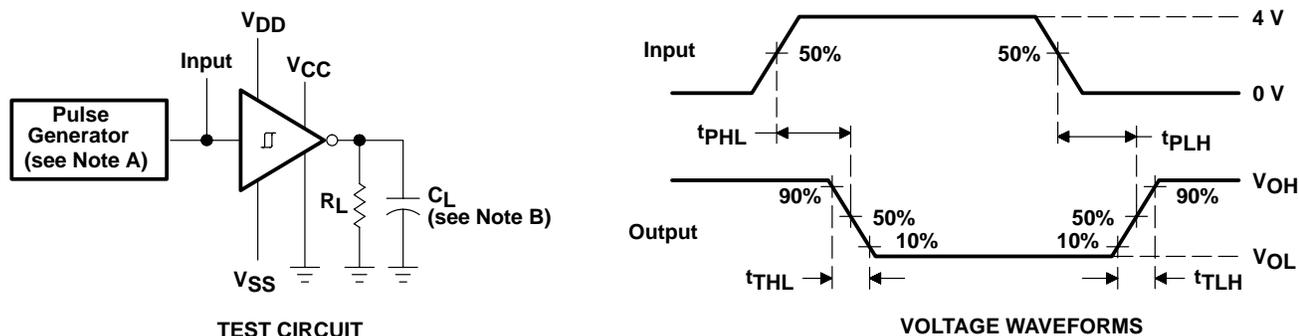
NOTES: A. The pulse generator has the following characteristics:  $t_w = 25 \mu s$ ,  $PRR = 20 \text{ kHz}$ ,  $Z_O = 50 \Omega$ ,  $t_r = t_f < 50 \text{ ns}$ .
