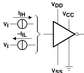
Figure 2. Driver Test Circuit ( $I_{IL}$ ,  $I_{IH}$ )
