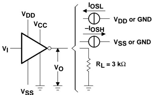
Figure 1. Driver Test Circuit ( $V_{OH}$ ,  $V_{OL}$ ,  $I_{OS(L)}$ ,  $I_{OS(H)}$ )
