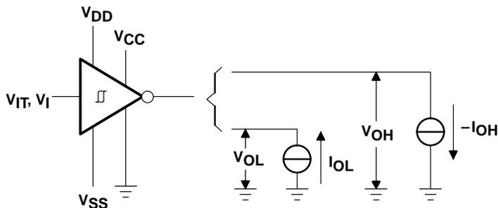
Figure 5. Receiver Test Circuit,  $V_{IT}$ ,  $V_{OL}$ ,  $V_{OH}$
