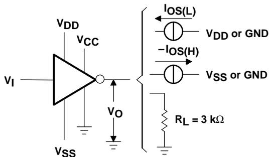
Figure 1. Driver Test Circuit
