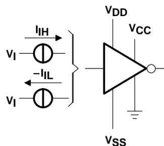
Figure 2. Driver Test Circuit,  $I_{iL}$ ,  $I_{iH}$
