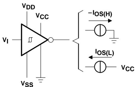
Figure 4. Receiver Test Circuit,  $I_{OS(H)}$ ,  $I_{OS(L)}$
