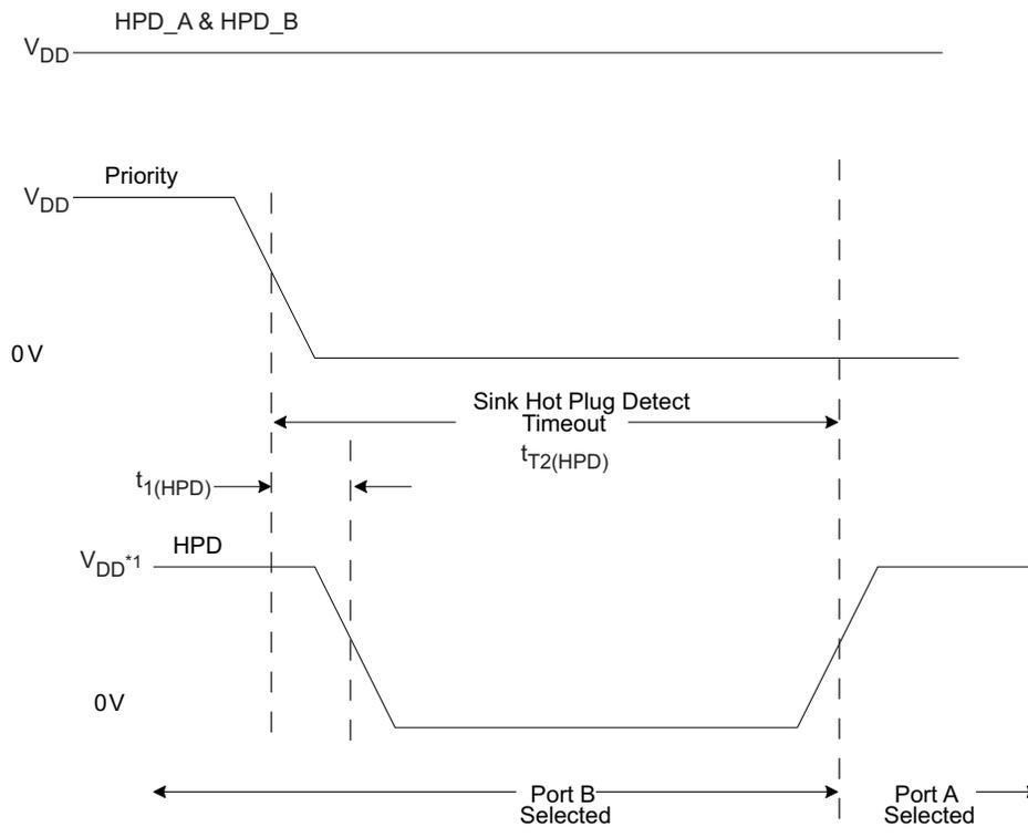
Figure 3. HPD Timing Diagram #2
