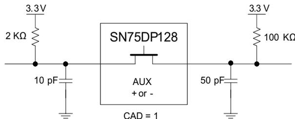
Figure 6. Auxiliary Channel Test Circuit (CAD = HIGH)
