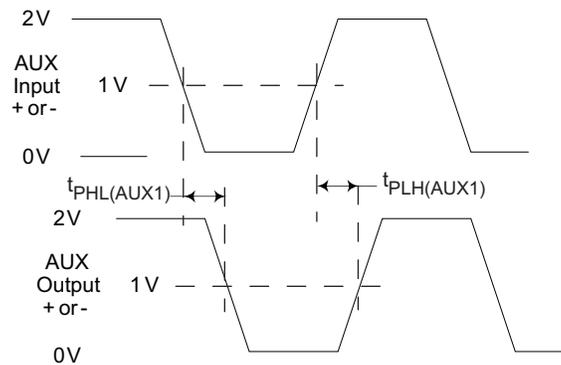
Figure 9. Auxiliary Channel Delay Measurement (CAD = HIGH)
