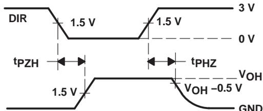
Figure 10. Receiver Enable/Disable Test, High Output
