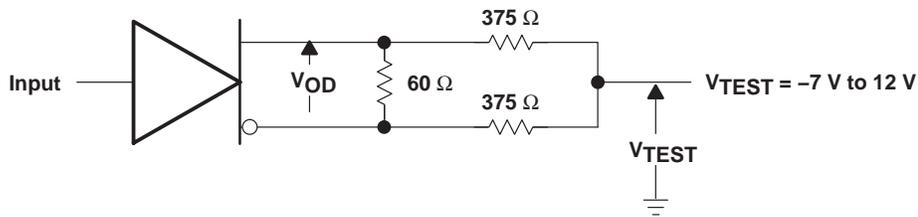
Figure 2. Driver Test Circuit,  $V_{OD}$  With Common-Mode Loading
