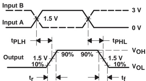
Figure 9. Receiver Switching Test Circuit and Waveforms
