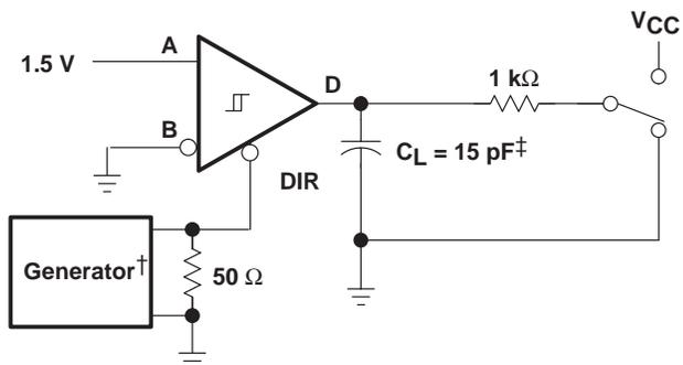
† PRR = 1 MHz, 50% Duty Cycle,  $t_r < 6$  ns,  $t_f < 6$  ns,  $Z_0 = 50 \Omega$
