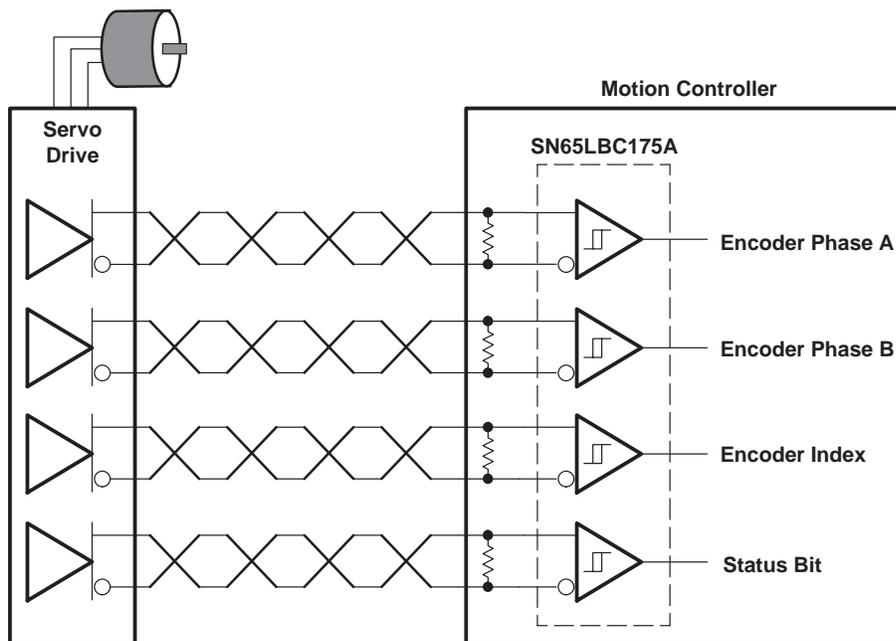
Figure 12. Typical Application Circuit, High-Speed Servomotor Encoder Interface
