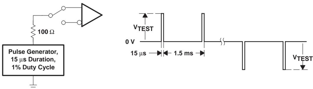
Figure 5. Test Circuit and Waveform, Transient Over-Voltage Test
