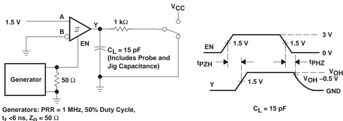
Figure 3. Test Circuit Waveforms,  $t_{PZH}$  and  $t_{PHZ}$
