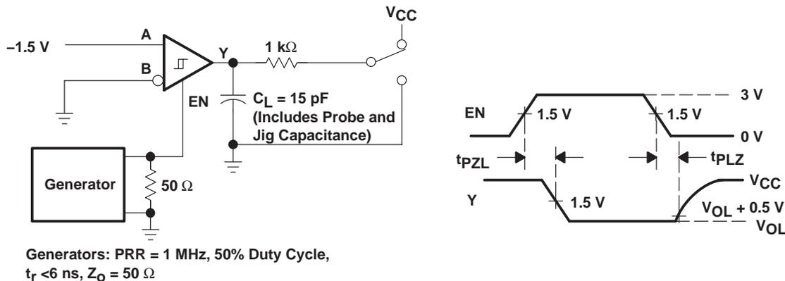
Figure 4. Test Circuit Waveforms,  $t_{pZL}$  and  $t_{pLZ}$
