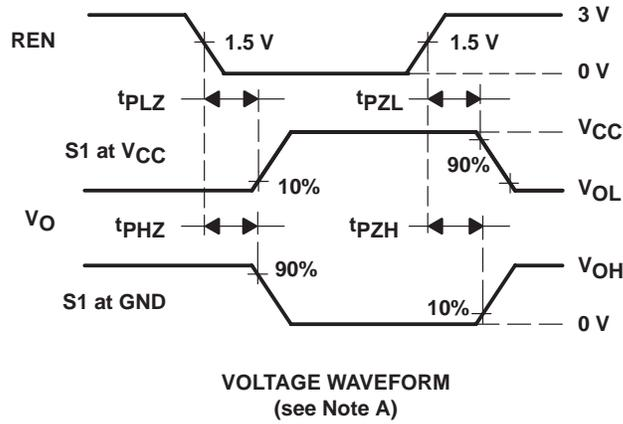
NOTE A: For the input waveform  $t_r, t_f \leq 10$  ns
