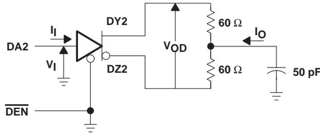
Figure 2. Differential Driver DC Parameter Test Circuit
