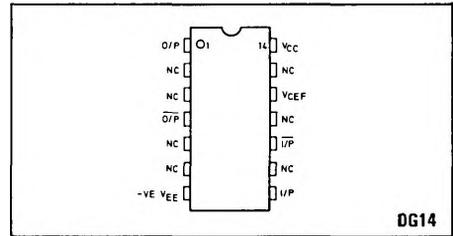
Fig. 1 Pin connections
