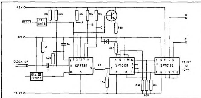
Fig.7 600MHz ÷ 32 with reset and inhibit
