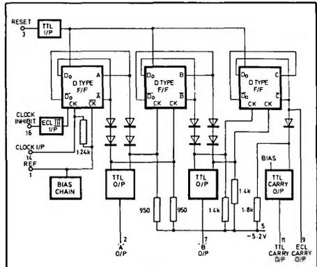
Fig. 2 SP8735/6 logic diagram
