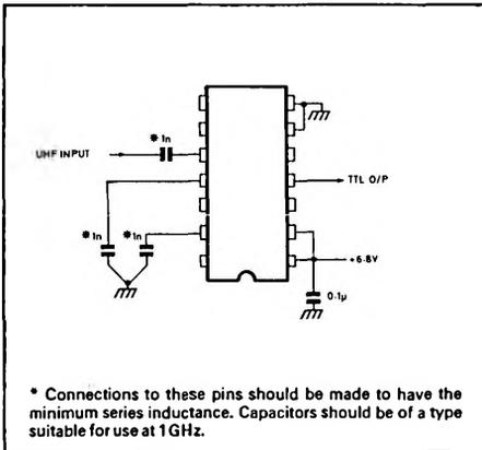
Fig. 3 Application circuit
