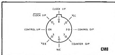
Fig. 1 Pin connections
