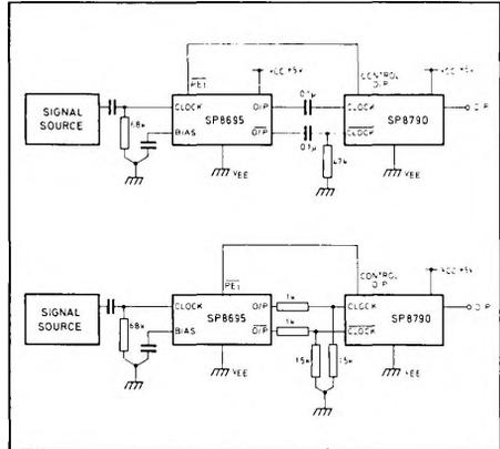
Fig. 6 Methods of preventing self-oscillation
