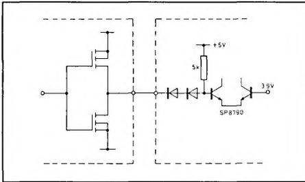
Fig. 3 CMOS and TTL compatible control input
