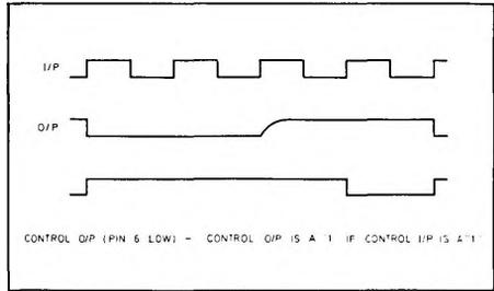
Fig. 4 SP8790 waveforms
