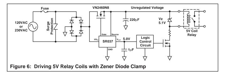
The circuit shown in Figure 6 uses the SR037 to supply a regulated 5.0V for the logic control circuitry. A 5.1V Zener diode is used in parallel with the 5.0V relay coil to ensure that the relay coil's maximum operating voltage is not exceeded. The Zener
